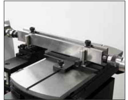
Comparative checking of gauge blocks > 250 mm (TA-SU-307/TEL7/TELM7)
