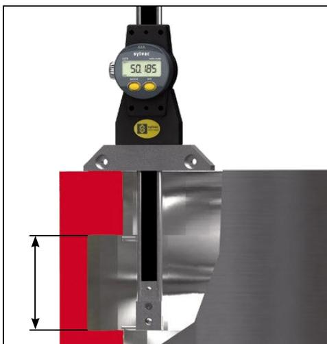
Measure of an internal groove (height) thanks to the constant.
