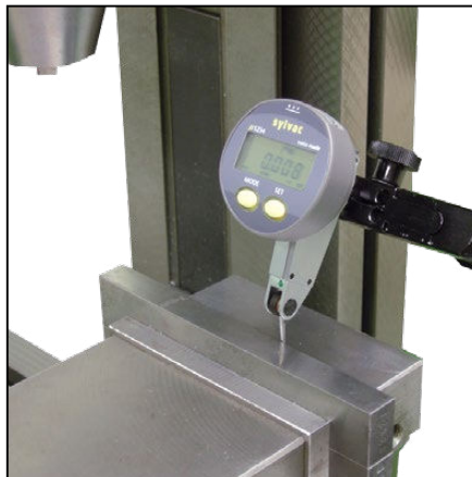
Checking the alignment on milling machine.
