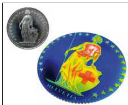
Measurement of macroscopic surface textures (CCM P1)
