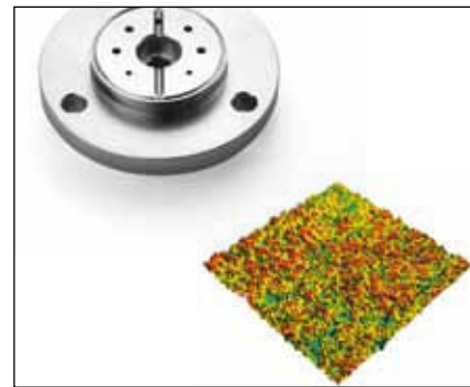
Texture analysis of a chemically polished titanium surface (DHM S2)
